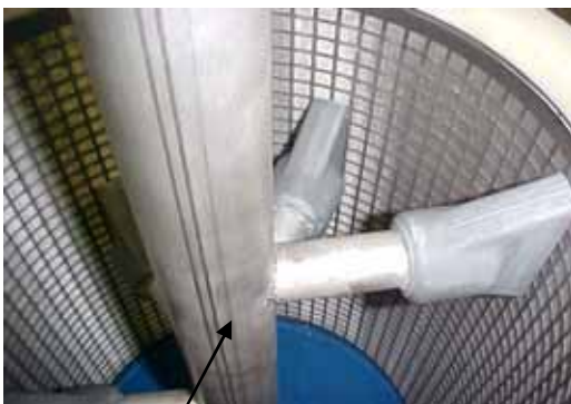
the electrical motor rotates the cleaning axle
