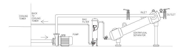
Water flows from the cooling tower to the centrifugal separator, by the main pump. Two alternatives are available for purging the separator :
